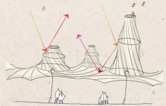
To solve the dynamic structure, achieving a constant protection from the sun, we developed a translational surface with a rigid axis, to make it look like an hyperbolic structure.
